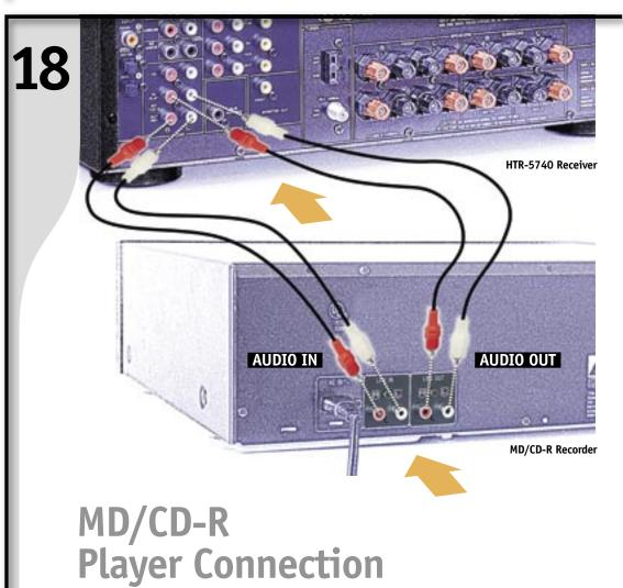
**Connect MD/CD-R Recorder (optional)** Connect RCA audio cables (not included) to "MD/CD-R" terminals on receiver as shown.
