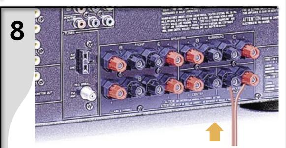
Connect Surround Back Speaker Positive (+) side of the wire with white stripe attaches to (+) terminal. Negative (-) side attaches to (-) terminal.
