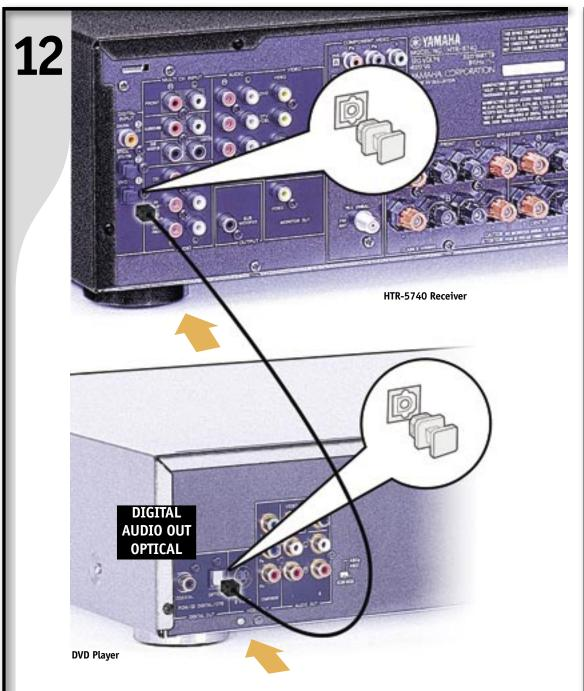
**DVD Player Optical Connection (optional)** Remove dust cap on optical input as shown on insets. Connect optical cable (not included) to receiver. Connect optical cable to DVD player (not included) from receiver.
