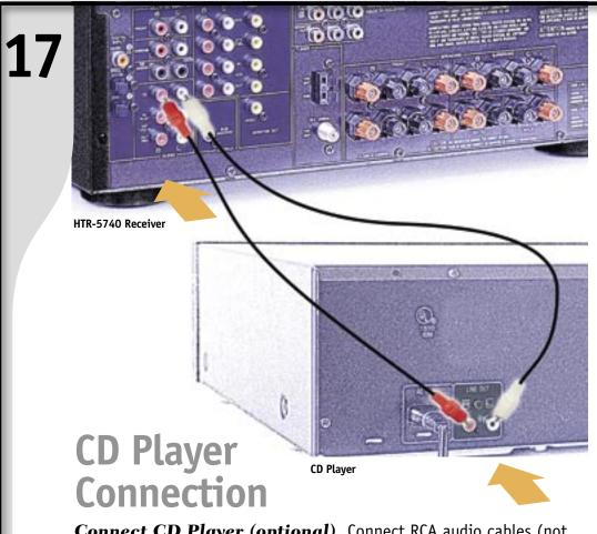
**Connect CD Player (optional)** Connect RCA audio cables (not included) to "CD" terminals on receiver as shown. If your CD Player has digital output terminal, connect digital cable (not included) to HTR-5740 Receiver Digital Input terminal. See page 17 of your HTR-5740 Owner's Manual for more information.
